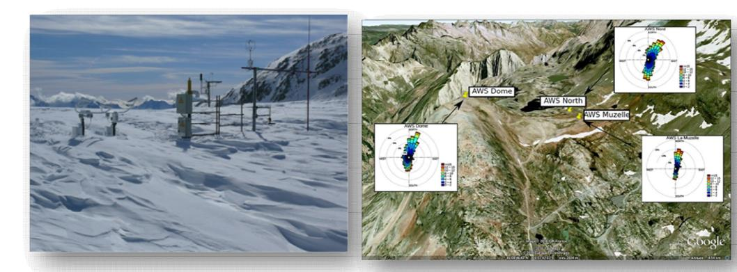
Automatic weather stations and drifting snow measurement inter-comparison at Col du Lac Blanc, French Alps.
