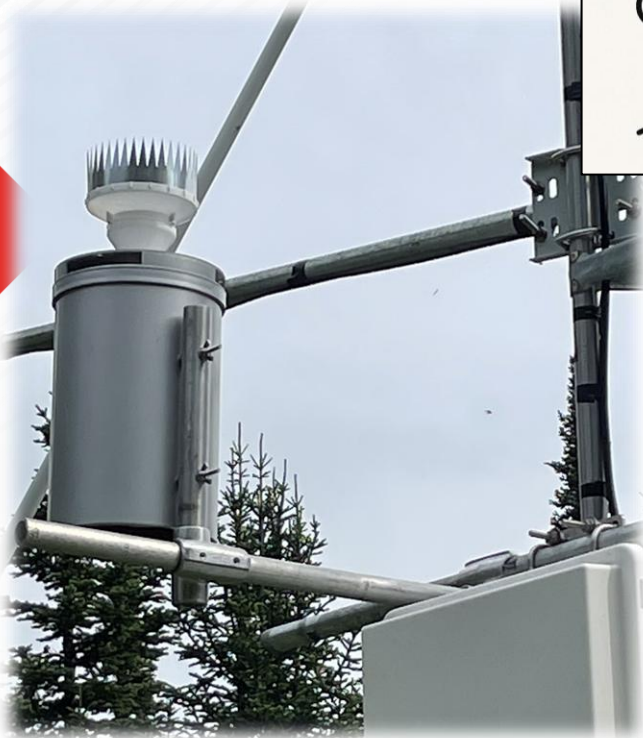
RS-1C Rainfall Sampler (Palmex)
