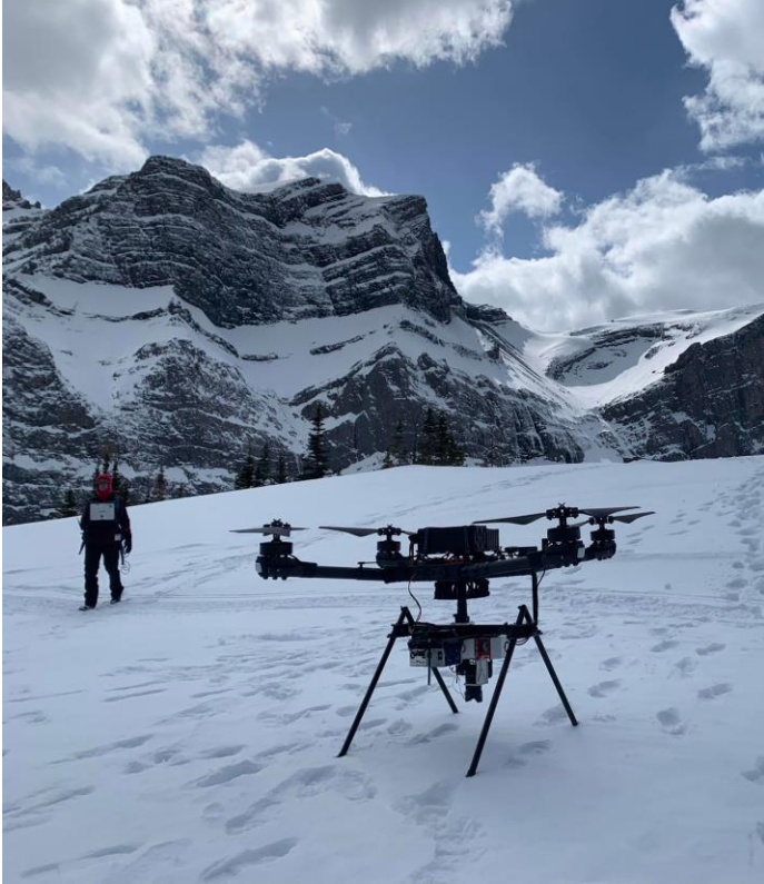
Alta-X mounted Reigl miniVUX-2 lidar used to collect surface elevation data over whole basin area
